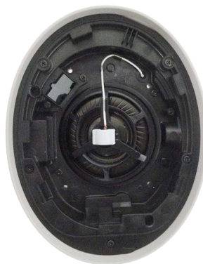
front plate portion (L-ch)
